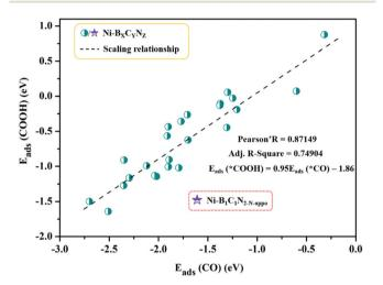
Fig. 4 Scaling relationship between the adsorption energies of \*COOH ( $E_{ads}(*COOH)$ ) and \*CO ( $E_{ads}(*CO)$ ).
