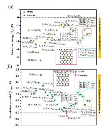
Fig. 1 The DFT-computed formation energy (a) and dissolution potential (b) of  $Ni-B_XC_YN_Z$  (X + Y + Z = 4). The inset shows the top view of the catalyst model, where the highlighted vellow atoms represent the coordination atoms of the Ni center (purple atom).
