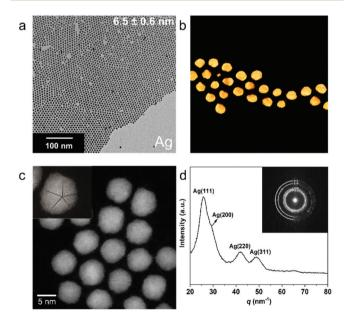
Fig. 2 (a) TEM image of colloidal Ag NPs. (b) 3D visualization of the reconstructed volume of a number of Ag NPs. (c) High resolution HAADF-STEM image of Ag NPs, showing the polycrystallinity of the NPs and the presence of pentatwinned domains. A magnified image of a region with a pentatwinned domain is shown as inset. (d) Fourier transform (FT) pattern (inset) of Aq NPs and the radially integrated 1D Powder Electron Diffraction (PED) pattern.
