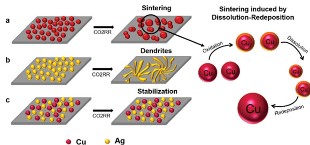
Fig. 8 Schematic illustration of the structural evolution of (a) Cu, (b) Ag and (c) Cu–Ag NP electrodes under electrochemical CO 2 RR conditions (−0.8 V vs. RHE), and the observed stabilization effect in binary Cu–Ag nanoparticle electrodes.
