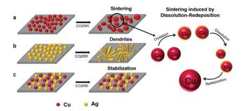
Fig. 8 Schematic illustration of the structural evolution of (a) Cu, (b) Ag and (c) Cu–Ag NP electrodes under electrochemical CO $_2$ RR conditions (–0.8 V vs. RHE), and the observed stabilization effect in binary Cu–Ag nanoparticle electrodes.
