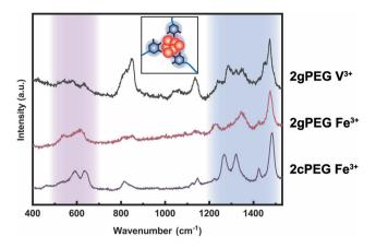
Fig. 5 Raman characterization of 2gPEG hydrogels. Resonance Raman spectra of 2gPEG crosslinked with V3+ and Fe3+, and 2cPEG crosslinked with Fe<sup>3+</sup>. The peaks between 500 and 680 cm<sup>-1</sup> are attributed to the catechol-Fe<sup>3+</sup> coordination or pyrogallol-Fe<sup>3+</sup> coordination, while the peaks between 1230 and 1500 cm<sup>-1</sup> are due to the carbon ring vibration
