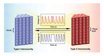
Fig. 25 Illustration of the fabrication process of AAO microcavities by pulse anodization. Type I microcavities are prepared by inserting a cavity layer between the AAO-DBR structures (left side in blue). Type II microcavities are fabricated by shifting the phase of anodization to achieve the phase modulation of an effective refractive index in the bottom Bragg reflector structure (right side in red). Reprinted with permission from ref. 363. Copyright © 2015, the American Chemical Society.
