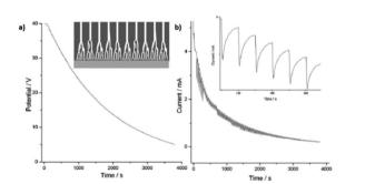
Fig. 10 (a) Potential-time and (b) current-time transients profiles recorded in non-steady-state anodization. Inset in (a) is a schematic illustration of the tree-like branched pores. Inset in b is the magnification of the current curve for a clear view of its tooth-like profile. Reprinted with permission from ref. 209. Copyright © 2007, The Royal Society of Chemistry.
