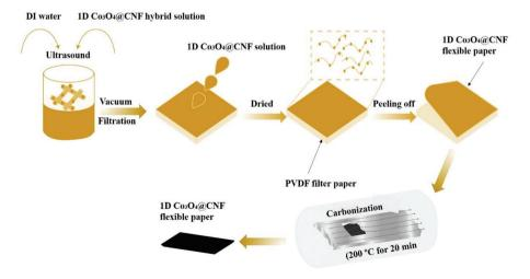
$\textbf{Scheme 1} \quad \text{Schematic vacuum filtration preparation of the 1D Co}_3O_4 @ \text{CNF flexible paper electrode}. \\$
