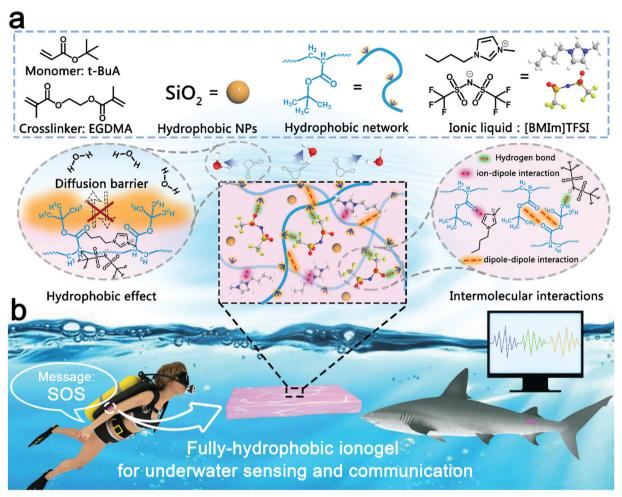
Fig. 1 Schematic of fabricating the fully hydrophobic ionogel for underwater sensors and communicators, (a) Structure of the fully hydrophobic ionogel (b) Potential applications in underwater sensing and underwater communication.
