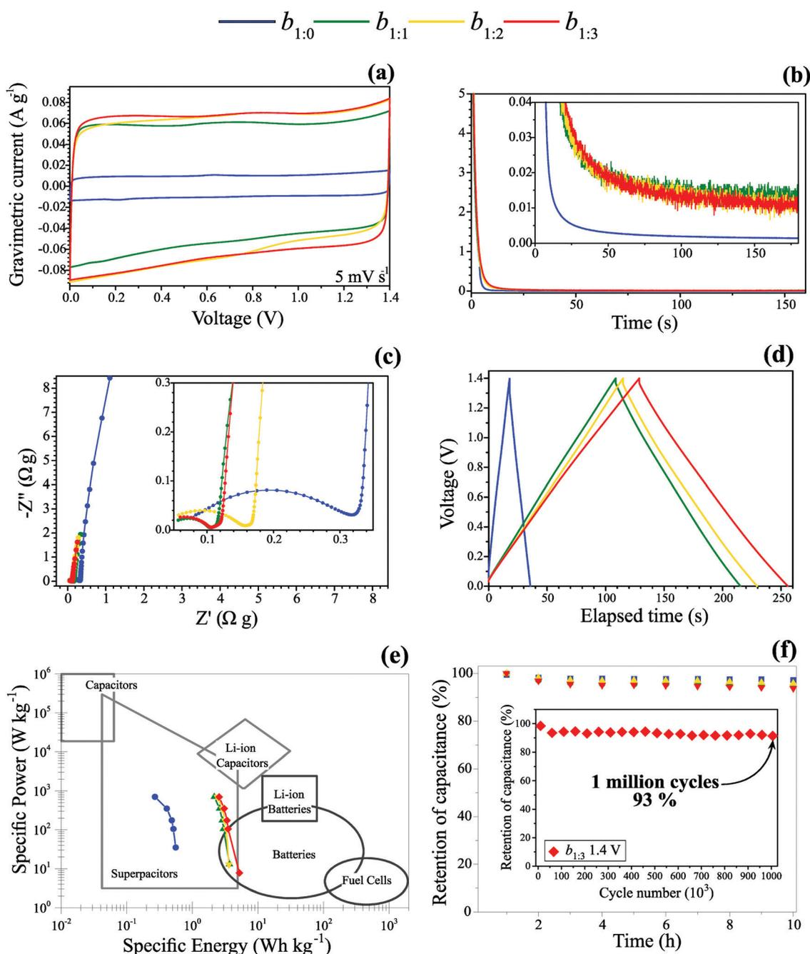
**Fig. 5** Electrochemical data and performance of the symmetric coin cell as a function of the MWCNT:AC mass ratio: (a) cyclic voltammograms at  $5 \text{ mV s}^{-1}$ , (b) transient currents during the SSC experiments at  $1.4 \text{ V}$ , (c) EIS at  $1.4 \text{ V}$ , (d) GCD at  $0.15 \text{ A g}^{-1}$ , (e) the Ragone plot, and (f) capacitance retention after 1 million cycles. Electrolyte:  $1.0 \text{ mol dm}^{-3} \text{ Li}_2\text{SO}_4$ .
