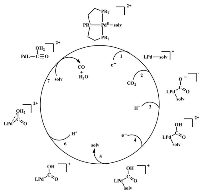
Scheme 6 General mechanistic scheme for the electrocatalytic CO<sub>2</sub> reduction by [Pd(triphosphine)(S)]<sup>2+</sup> catalysts.
