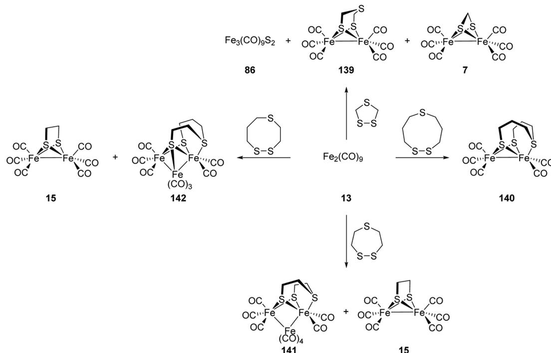
Fig. 41 Syntheses of multi-metallic complexes from sulphur heterocycles.
