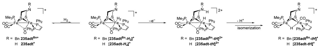
Fig. 84 Hydrogen oxidation by complexes **235adt**<sup>R+</sup>.
