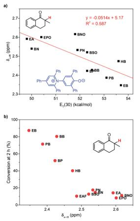
Fig. 4 (a) Correlated chemical shift of the  $\alpha$ -proton in  $\bf 1$  with the  $E_T(30)$  value in 1-alkyl-3-methylimidazolium ILs. (b) The relationship between the conversion of  $\bf 1$  at 2 h and the chemical shift of the  $\alpha$ -proton in  $\bf 1$ .
