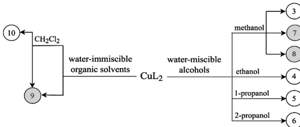
**Scheme 2** Crystallization experiments used to obtain crystals 3–10. Compound numbers with white background: crystals which enclathrate solvents; compound numbers with grey background: different polymorphic forms of  $\text{CuL}_2$ .
