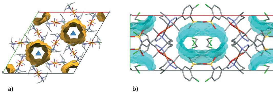
Fig. 13 (a) Empty channels in the crystal structure of **9** viewed from the crystallographic *c* axis. The three-fold axes are shown as blue triangles. (b) Unit cell of crystal **10** viewed from the crystallographic *c* axis. The channels in the crystal lattice (highlighted by cyan) are filled by DCM molecules which are surrounded by four complex molecules.
