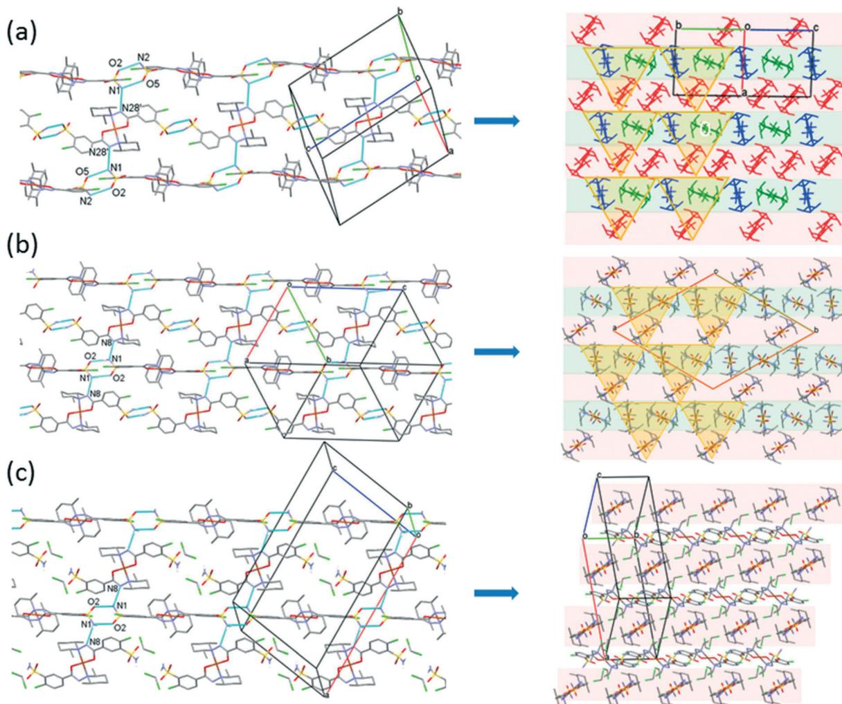
**Fig. 11** Packing arrangements in crystal **8** (a) (molecule A is red, B is green and C is blue), crystal **9** (b) and crystal **10** (c) showing the columns formed by N–H···O type hydrogen bonds viewed from the side and also from the top of the columns. The light pink and green colours show the different sheets; the yellow triangles highlight the triangular arrangements of the molecules in the different crystals.
