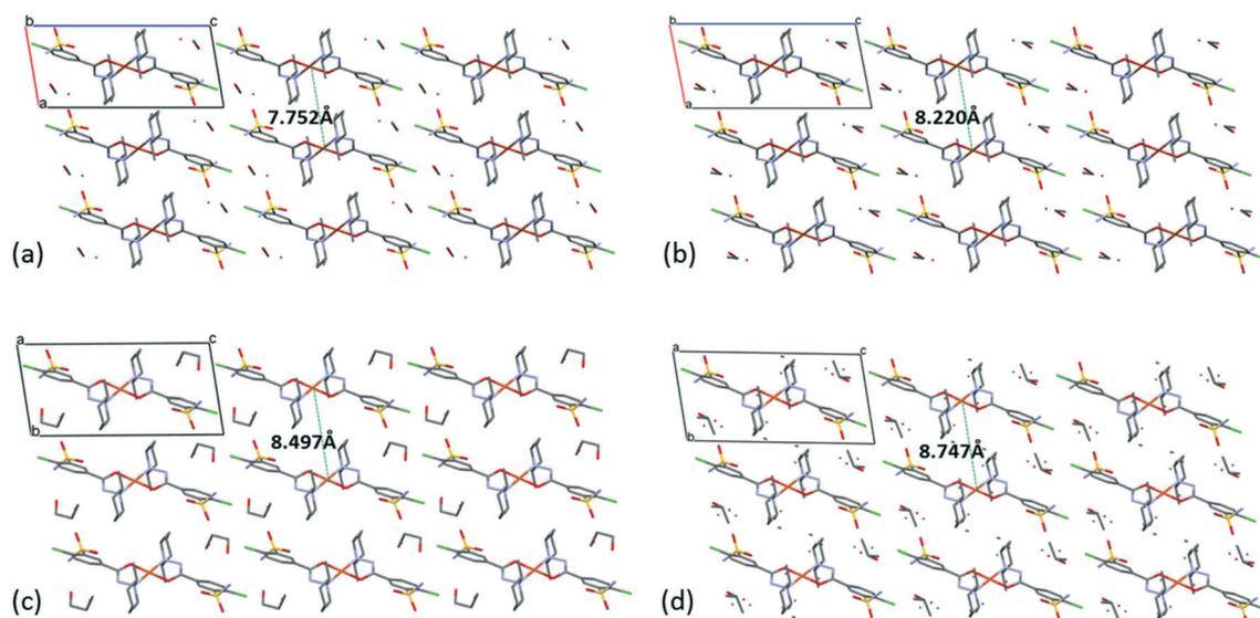
Fig. 5 Packing arrangements in crystal **3** (a), **4** (b), **5** (c) and **6** (d) viewed from the crystallographic *b* axis, presenting also the increasing distances of the metal Cu(II) centres with the increasing size of the solvent guest molecules.
