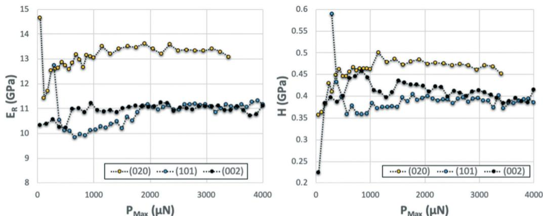
Fig. 6 Series of nanoindentation measurements carried out with increasing  $P_{\text{Max}}$  on three single crystals of CBZ oriented along the three different crystal directions. The derived  $E_{\text{R}}$  (left) and  $H$  (right) as a function of  $P_{\text{Max}}$  appear fairly constant across the entire range tested.
