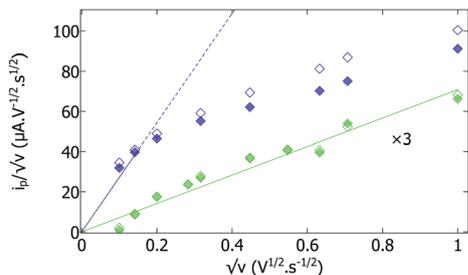
**Fig. 2** Evaluation of the thin (green, enlarged three times) and thick (dark blue) hydrogenase/polymer films by cyclic voltammetry under non-catalytic conditions (under argon). Plot of anodic (open) and cathodic (full) peak currents divided by the square root of scan rate ( $i_p/v$ ), against  $\sqrt{v}$ . A straight line through the origin is expected when the film is so thin that all viologen moieties are oxidized or reduced in each sweep.
