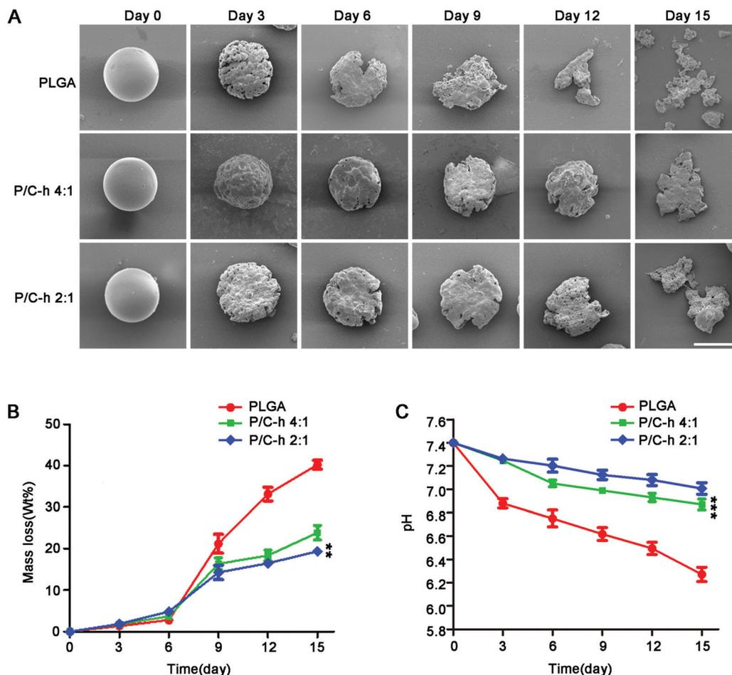
Fig. 3 Degradation properties of PLGA, P/C-h 4:1, and P/C-h 2:1 microparticles. (A) SEM images of the microparticles. Scale bars = 20  $\mu\text{m}$ . (B) Weight loss of microparticles immersed in PBS for 0, 3, 6, 9, 12 and 15 days. (C) The pH value changes of the solutions immersing the microparticles for 0, 3, 6, 9, 12 and 15 days. The data were reported as the mean  $\pm$  SD,  $n = 5$ . \*\*\* significant difference,  $p < 0.001$ . \*\* significant difference,  $p < 0.01$ .
