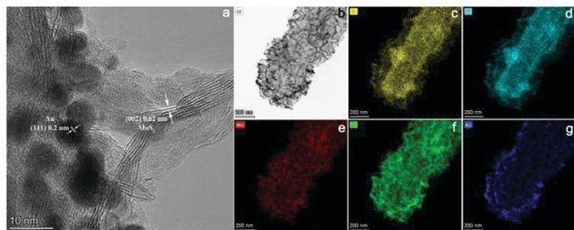
Fig. 3 The HRTEM image of PPy@MoS<sub>2</sub>@Au (a and b), and the corresponding elemental mapping images of C (c), N (d), Mo (e), S (f) and Au (g).
