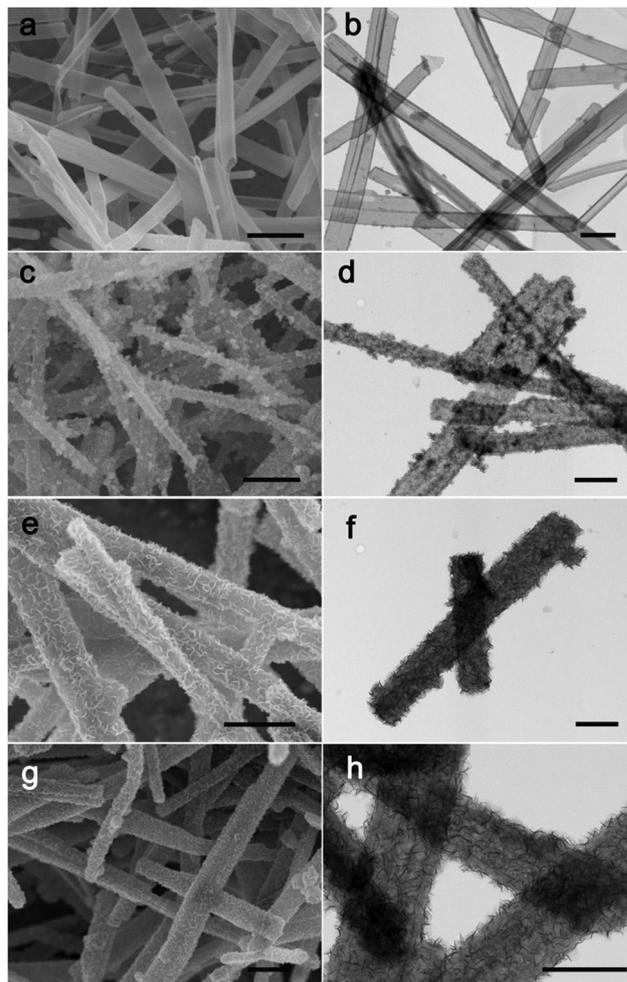
Fig. 6 SEM and TEM images of PPy@MoS<sub>2</sub>, 3 h (a and b), 6 h (c and d), 12 h (e and f) and 24 h (g and h). Scale bars: 1 μm in (a, c, e and g), and 500 nm in (b, d, f and h).
