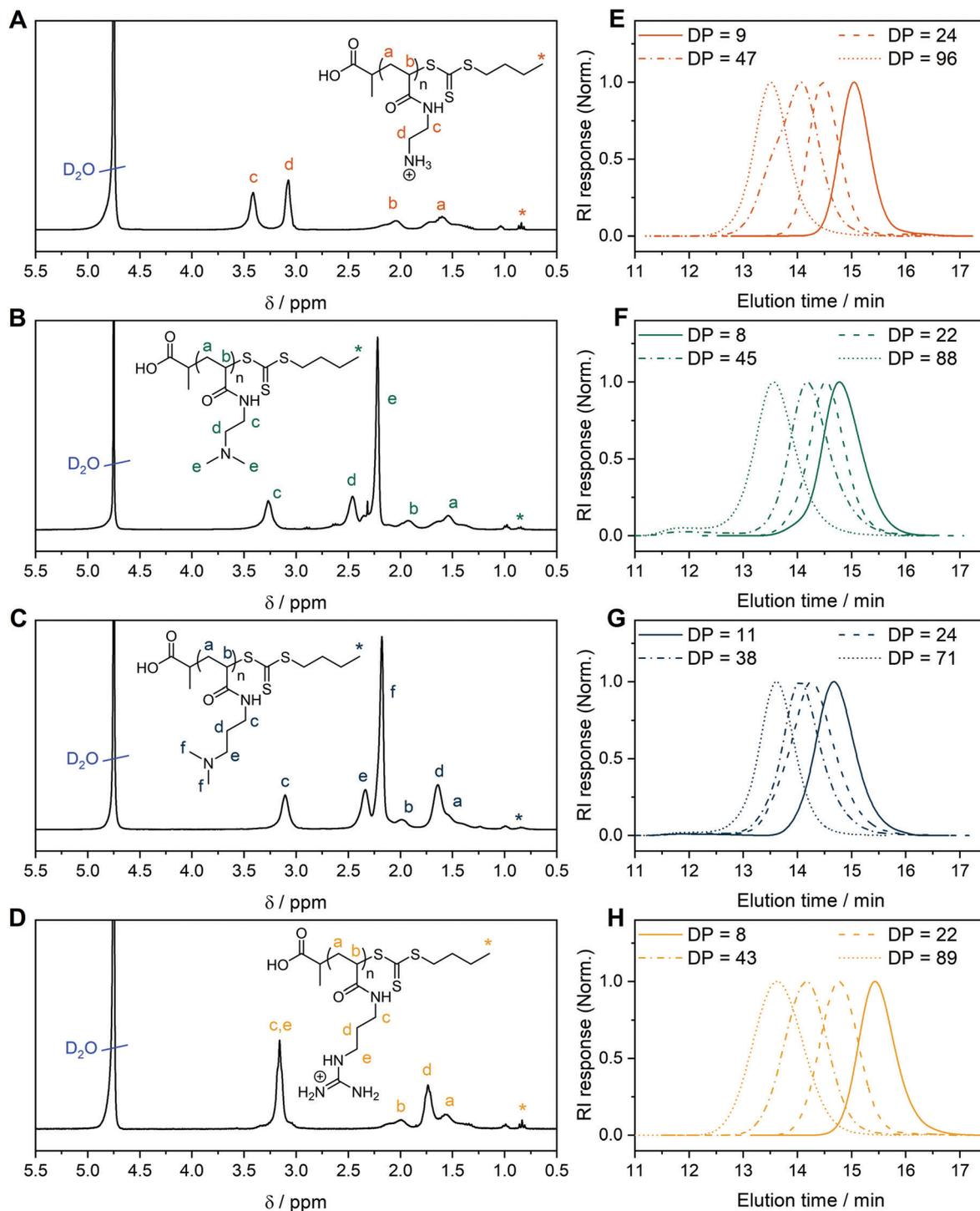
Fig. 1 <sup>1</sup>H NMR of (A) PAEAm<sub>24</sub>, (B) PDMAEAm<sub>22</sub>, (C) PDMAPAm<sub>24</sub>, (D) PGPAm<sub>22</sub> in D<sub>2</sub>O. Aqueous (0.1% TFA + 0.1 mol L<sup>-1</sup> NaCl) SEC traces of (E) PAEAm, (F) PDMAEAm, (G) PDMAPAm, (H) PGPAm polymers synthesized via RAFT polymerization.
