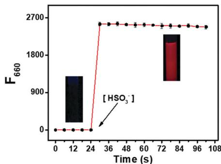
Fig. 2 Time course of the fluorescence response ( $F_{660}$ ) of DCQN (10  $\mu\text{M}$ ) to  $\text{HSO}_3^-$  (100.0  $\mu\text{M}$ ) in HEPES buffer solution (10 mM, pH 7.4, with 10% DMSO, v/v) at 25  $^\circ\text{C}$ . The excitation wavelength was 550 nm. Slits: 5/5 nm, the error bars represent  $\pm$  SD,  $n = 3$ .
