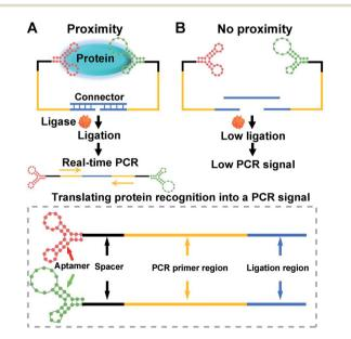
Scheme 1 Scheme of aptamer-assisted proximity ligation assay for COVID-19 antigens. (A) Probes that bind to the same protein target are in close proximity, initiating ligation-dependent qPCR amplification. (B) Unbounded probes that are not in proximity show low ligation efficiency, resulting in low PCR signal.
