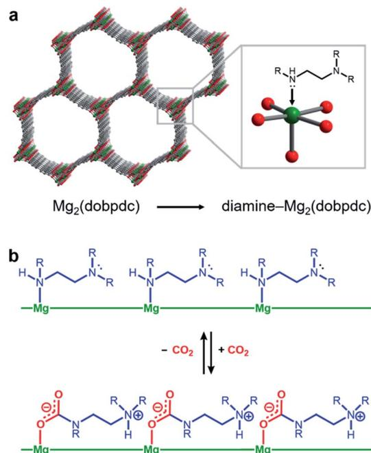
Fig. 1 Structure of diamine-appended variants of the metal–organic framework Mg<sub>2</sub>(dobpdc). (a) Diamines are appended post-synthetically to the open Mg<sup>2+</sup> sites of the framework. (b) Schematic representation of the resulting adsorbents capturing CO<sub>2</sub> cooperatively through the formation of ammonium carbamate chains.
