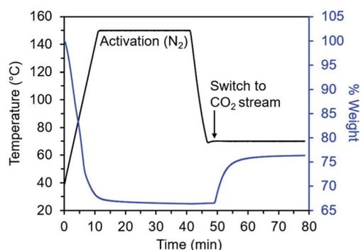
Fig. 2 Overview of TGA adsorption kinetics assay. The diamine-appended metal-organic framework sample is activated within a thermogravimetric analyzer under flowing  $\text{N}_2$  to remove solvent molecules and non-metal-bound diamines from the pores. The sample is then cooled under  $\text{N}_2$  to the temperature of interest, the gas flow is switched to a  $\text{CO}_2$ -containing stream, and  $\text{CO}_2$  adsorption is monitored as a function of time.
