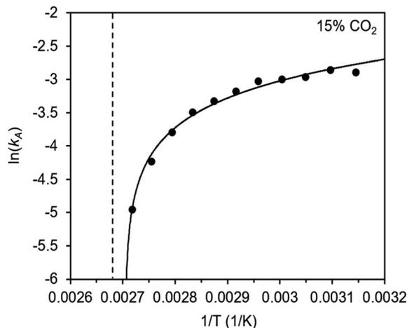
Fig. 8 Arrhenius plot for CO<sub>2</sub> adsorption from a 15% CO<sub>2</sub> in N<sub>2</sub> stream by m-2-m-Mg<sub>2</sub>(dobpdc). The dotted line indicates the step temperature under 15% CO<sub>2</sub>. The curved solid line represents a logarithmic fit to the data:  $y = 2.05 + 0.624 \ln(x - 0.0027)$ . Root mean square error (RMSE): 0.063. Range of the dependent variable: 2.198 (RMSE/range)  $\times 100\% = 2.9\%$ .
