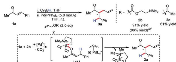
Scheme 3 Effect of leaving group on efficiency of ketone alkylation.<sup>a</sup> Yield for 10.0 mmol scale.
