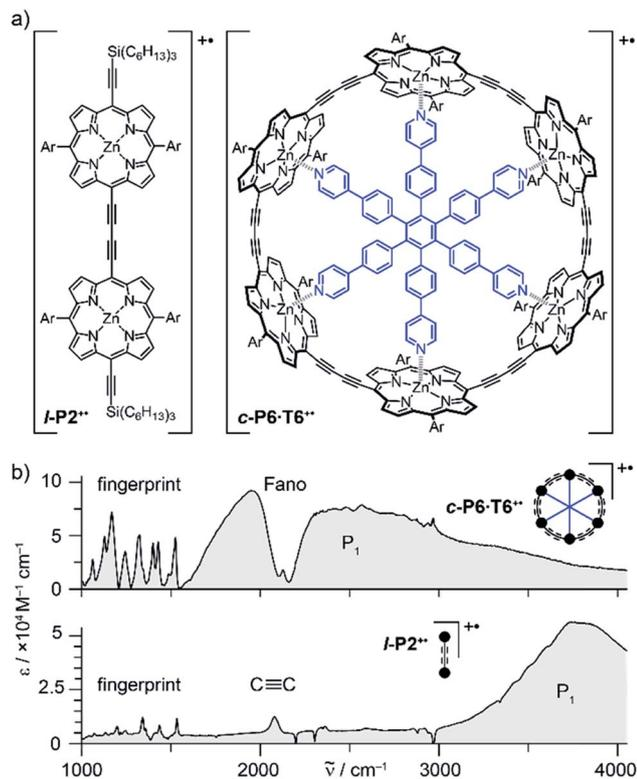
Fig. 1 (a) Chemical structures of the porphyrin oligomer radical cations  $l\text{-P}2^{2+}$  and  $c\text{-P}6\cdot\text{T}6^{2+}$ . Ar = 3,5-bis(trihexylsilyl)phenyl. (b) Their FTIR spectra recorded in  $\text{CD}_2\text{Cl}_2$  showing the fingerprint region, the  $\text{C}\equiv\text{C}$  stretch band, the Fano anti-resonance (for  $c\text{-P}6\cdot\text{T}6^{2+}$ ) and the  $\text{P}_1$  polaron band.
