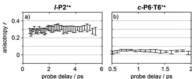
Fig. 6 Average anisotropy of all analyzed signals (greyed areas in Fig. 5a and b) of  $I\text{-P2}^{+\bullet}$  (a) and  $c\text{-P6}\cdot\text{T6}^{+\bullet}$  (b) pumped both at  $2100\text{ cm}^{-1}$  and  $3250/2500\text{ cm}^{-1}$  as a function of probe time delay.
