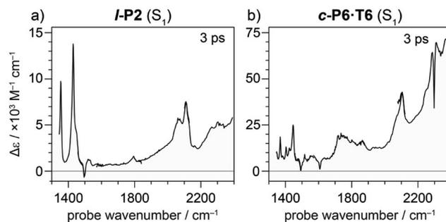
Fig. 7 TRIR spectrum at 3 ps delay of neutral molecules (a)  $I\text{-P2}$  and (b)  $c\text{-P6}\cdot\text{T6}$  excited to  $S_1$  excited state with visible light (714 nm and 772 nm, respectively). Strong ESA and weak or absent GSB is observed suggesting the presence of IRAVs in the  $S_1$  excited states of neutral molecules.
