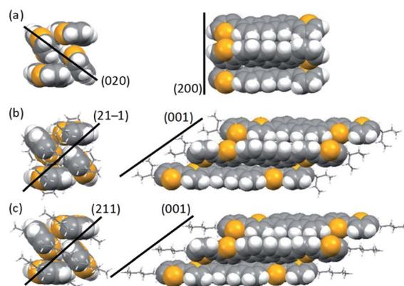
Fig. 5 Molecular packing in single crystals of (a) DTA,<sup>25</sup> (b) EBDBTA, and (c) C6DBTA. Left and right columns are views along and normal to the long molecular axis, respectively. Black lines indicate approximate positions of the crystal planes relevant to the slipped or non-slipped herringbone motifs.
