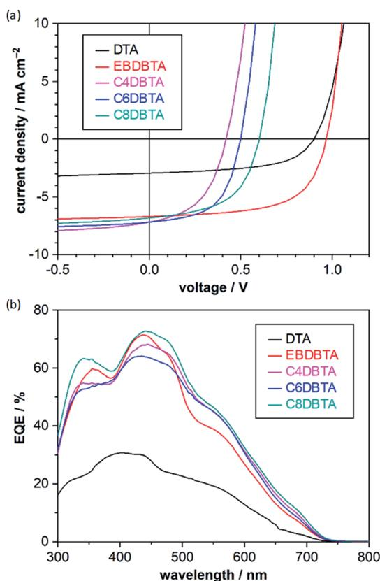
Fig. 3 Photovoltaic response of the p-i-n OPVs. (a)  $J$ - $V$  curves; (b) EQE spectra. Data are of the best-performing cells in each entry shown in Table 1. The  $J$ - $V$  measurements were performed under simulated AM1.5G illumination at 100 mW cm<sup>-2</sup>. Active-layer structure: [PhBADT/(DTA or RDBTA):PC<sub>71</sub>BM/PC<sub>71</sub>BM].
