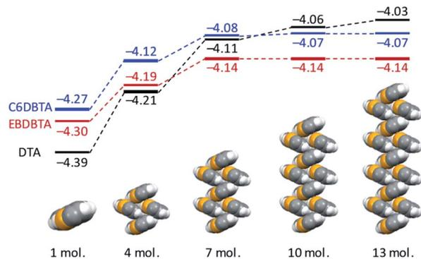
Fig. 6 Calculated HOMO energies for single and sets of molecules in the single-crystal X-ray structures of DTA,<sup>25</sup> EBDBTA, and C6DBTA. Calculations were performed at the PBE/PBE/6-31G(d) level of theory.
