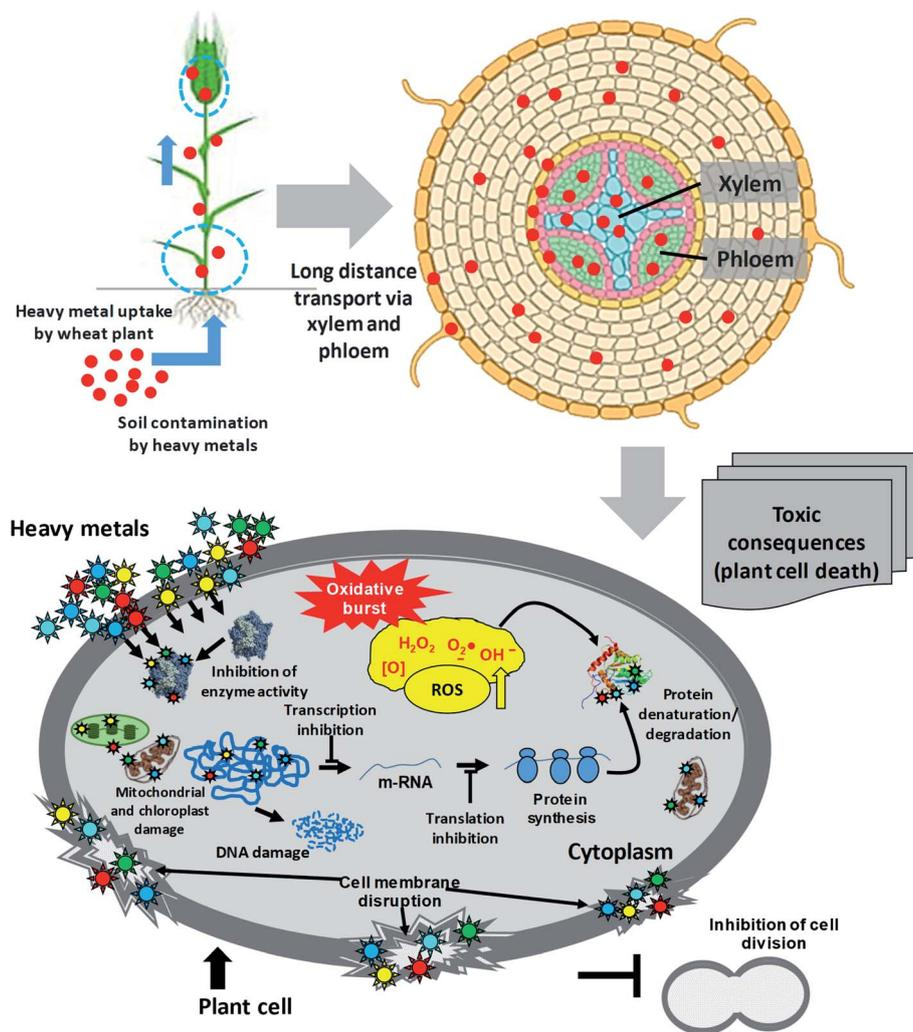
Fig. 2 Sequence of events from metal entry into a plant cell to the death of the plant.
