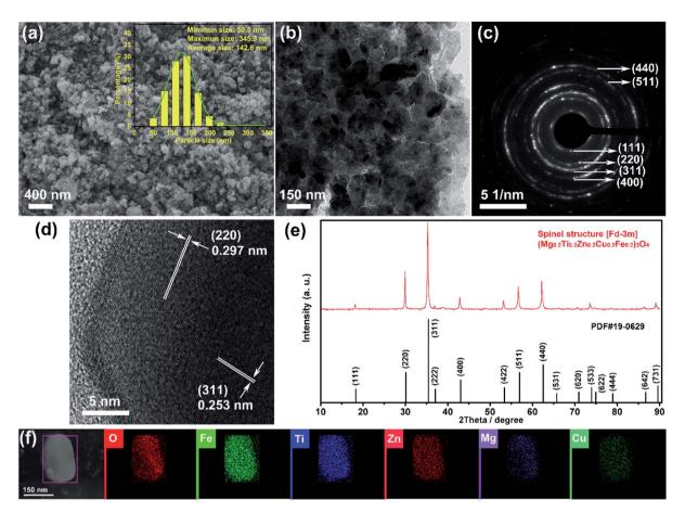
Fig. 1 (a) SEM image and (b) TEM image of the synthesized irregular  $(Mg_{0.2}Ti_{0.2}Zn_{0.2}Cu_{0.2}Fe_{0.2})_3O_4$  particles; (c) SAED pattern, (d) HR-TEM image, (e) XRD pattern and (f) elemental mapping images of the  $(Mg_{0.2}Ti_{0.2}Zn_{0.2}Cu_{0.2}Fe_{0.2})_3O_4$  particles.
