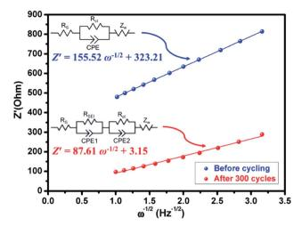
Fig. 3 Plots of Z' against  $\omega^{-1/2}$  (inset: equivalent circuit) of the fresh  $(Mg_{0.2}Ti_{0.2}Zn_{0.2}Cu_{0.2}Fe_{0.2})_3O_4$  half-cell and the half-cell charged to 3.0 V after 300 cycles.
