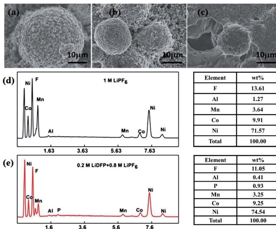
Fig. 8 SEM images of the NCM 811 electrode: fresh (a) and after 130 cycles in (b) the dual-salt electrolyte containing 0.8 M  $\text{LiPF}_6$  + 0.2 M LiDFP, (c) the blank electrolyte containing 1 M  $\text{LiPF}_6$ . The corresponding EDS analysis of surface element distribution of the NCM 811 electrode after 130 cycles in blank electrolyte (d) and dual-salt electrolyte (e).
