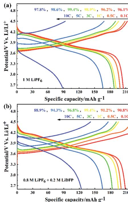
Fig. 4 The rate performance of NCM811/Li cells with (a) the blank electrolyte containing 1 M LiPF<sub>6</sub>; and (b) the dual-salt electrolyte containing 0.8 M LiPF<sub>6</sub> + 0.2 M LiDfP.
