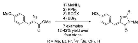
Scheme 15 Aza-Wittig reaction to produce 5-ethylidene-4-imidazolones.
