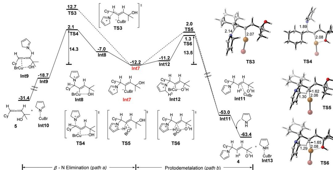
Fig. 2 Free energy profile ( $\Delta G$  in kcal mol<sup>-1</sup>) for either intramolecular protodemetalation or  $\beta$ -N elimination from Int7. Bond lengths are given in angstroms.
