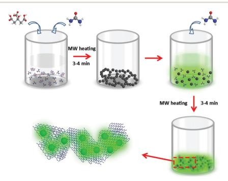
Fig. 1 Schematic representation of the synthesis of CDs@g-C<sub>3</sub>N<sub>4</sub> composites via a two-step microwave-assisted in situ heating method using citric acid and urea as precursors in water (MW: microwave)
