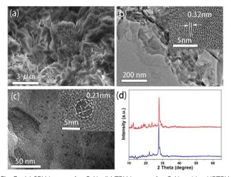
Fig. 3 (a) SEM image of  $g-C_3N_4$ . (b) TEM image of  $g-C_3N_4$ , with a HRTEM image shown in the inset. (c) TEM image of a CDs@g-C<sub>3</sub>N<sub>4</sub> composite with 1 wt% CDs, with a HRTEM image in the inset. (d) XRD patterns of bare  $g-C_3N_4$  (red line) and the CDs@g-C3N4 composite with 1 wt% CDs (blue line).
