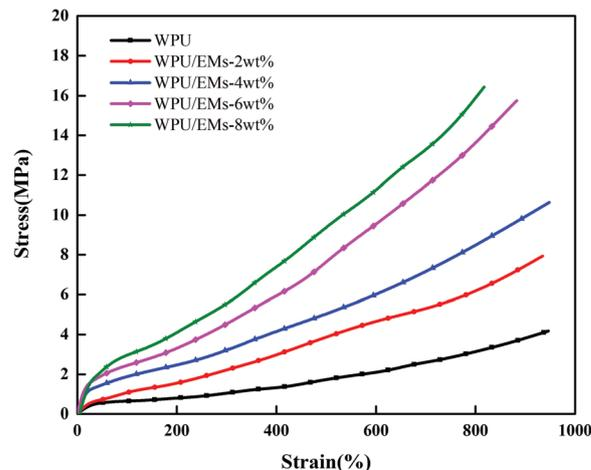
Fig. 8 Tensile testing curves of WPU and WPU/Ems composite films.
