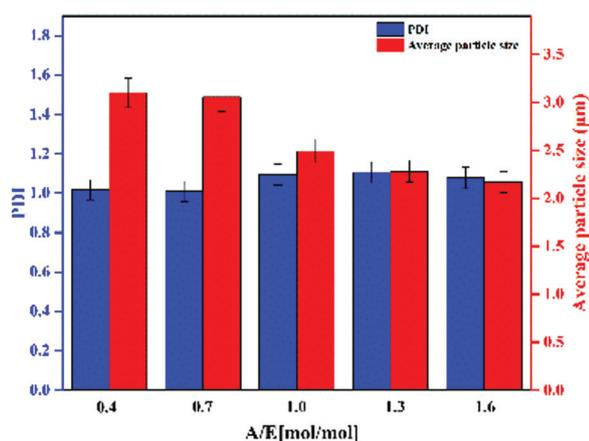
Fig. 3 PDI and average particle size of Ems.
