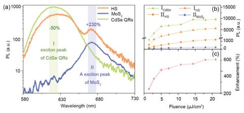
Fig. 2 (a) PL spectra of heterostructure (orange), pristine MoS<sub>2</sub> monolayer (blue), and CdSe QRs (green). (b) PL intensity of all of the heterostructure,  $MoS_2$ , and CdSe QRs. (c) PL enhancement of  $MoS_2$  as a function of incident fluence. Defining  $II_{HS}/II_{MoS_2}$  as PL enhancement
