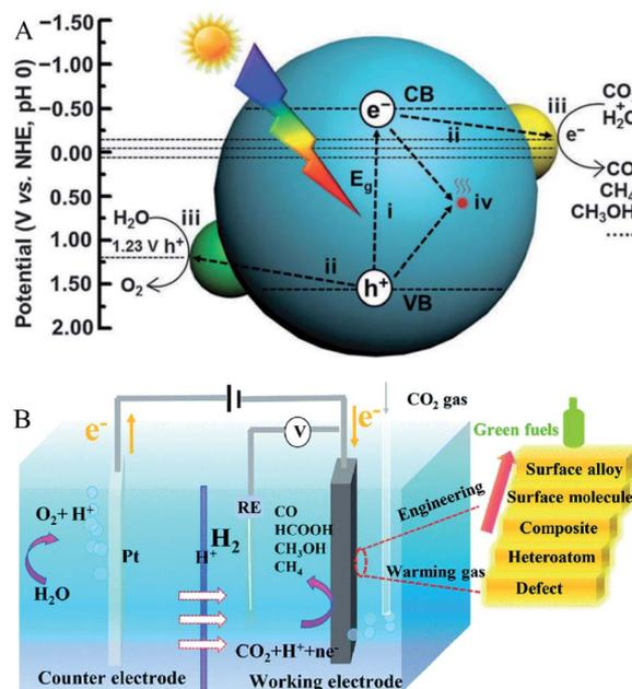
Fig. 1 (A) Schematic illustration of CO<sub>2</sub> photoreduction. Reproduced with permission: Copyright The Royal Society of Chemistry 2016;<sup>16</sup> (B) schematic illustration of CO<sub>2</sub> electroreduction. Reproduced with permission: Copyright The Royal Society of Chemistry 2019.<sup>17</sup>
