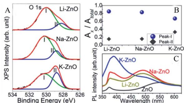
Fig. 5 High-resolution XPS spectra of (A) O 1s for the doped ZnO NRs, (B) the peak area ratios of peak-I and peak-II to the total area, (C) room-temperature PL emission peak spectra of the alkali metal doped ZnO NRs. Reproduced with permission: Copyright 2018 Wiley-VCH Verlag GmbH & Co. KGaA, Weinheim.<sup>41</sup>
