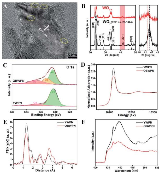
Fig. 4 (A) HRTEM image of OBWPN, (B) XRD patterns of YWPN (black) and OBWPN (red), (C) O 1s XPS spectra of YWPN and OBWPN, (D) normalized W  $L_{3}$ -edge XANES spectra of YWPN and OBWPN, (E) fourier transform (FT) of k-weighted W EXAFS spectra of YWPN and OBWPN, (F) photoluminescence spectra of YWPN and OBWPN. Reproduced with permission: Copyright 2018 Elsevier Inc.<sup>39</sup>
