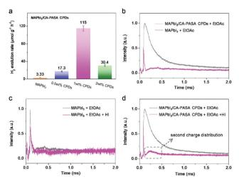
Fig. 3 Photocatalytic performance and mechanism. (a) Rate of  $H_2$  evolution over MAPbl<sub>3</sub> hybrids with different CPD contents. (b) *In situ* TPV curves of MAPbl<sub>3</sub> and CA-PASA CPDs covered with EtOAc. *In situ* TPV curves recorded with (c) MAPbl<sub>3</sub> and (d) CA-PASA CPD/MAPbl<sub>3</sub> working electrodes in 1 vol% HI/EtOAc mixed solution (v/v).
