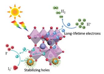
Scheme 1 Schematic diagram of the photocatalytic mechanism for CA-PASA CPDs/MAPbl3.
