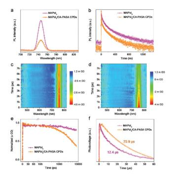
Fig. 2 Enhanced charge separation and lifetime in MAPbI<sub>3</sub>/CA-PASA CPDs. (a) Steady-state PL and (b) TRPL spectra of MAPbI<sub>3</sub> and MAPbI<sub>3</sub>/ CPDs. (c) MAPbl<sub>3</sub> and (d) MAPbl<sub>3</sub>/CPD spectro-temporal TA maps excited at 400 nm. (e) Characteristic dynamics for MAPbl<sub>3</sub> and MAPbl<sub>3</sub>/CPDs probed at 760 nm. (f) TPV curves of MAPbl<sub>3</sub> and MAPbl<sub>3</sub>/CPDs under 355 nm excitation. All hybrid samples contain 1 wt% CPDs.
