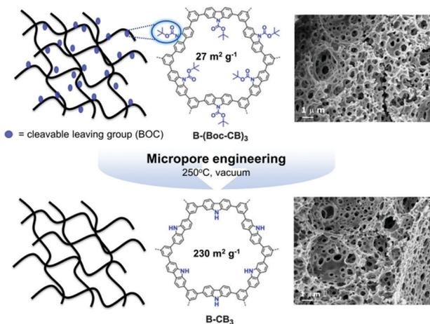
Fig. 19 Porosity control of CPPs by thermal deprotection of the functional group. Generation of additional porosity via a thermal deprotection of the BOC group in  $\pi$ -conjugated polyHIPEs. Reproduced with permission.<sup>23</sup> Copyright 2014 The Royal Society of Chemistry.
