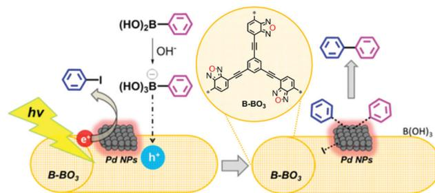
Fig. 15 Organic/inorganic hybrid structure of CPPs for electron transfer. Heterojunction formation between poly(benzoxadiazole) and palladium nanoparticles. Reproduced with permission.<sup>112</sup> Copyright 2015 American Chemical Society.
