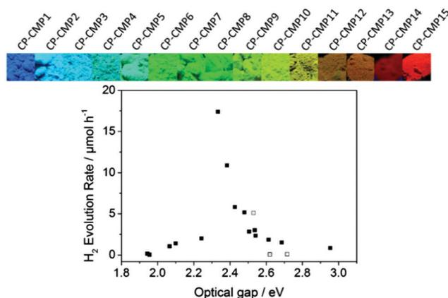
**Fig. 4** Statistical copolymerization of comonomers for band gap engineering of CPP. Pyrene-based conjugated microporous polymers and their photocatalytic  $\text{H}_2$  production efficiencies. Reproduced with permission.<sup>28</sup> Copyright 2015 American Chemical Society.
