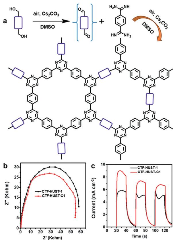
Fig. 9 Crystallinity of CPPs for charge transport. (a) Synthetic scheme of crystalline CTF-HUST-1 through *in situ* formation of aldehyde monomer from alcohol monomer. (b) Electrochemical impedance spectroscopy Nyquist plots and (c) photocurrent responses of the crystalline CTF-HUST-C1 and the layered CTF-HUST-1. Reproduced with permission.<sup>95</sup> Copyright 2018 Wiley-VCH.
