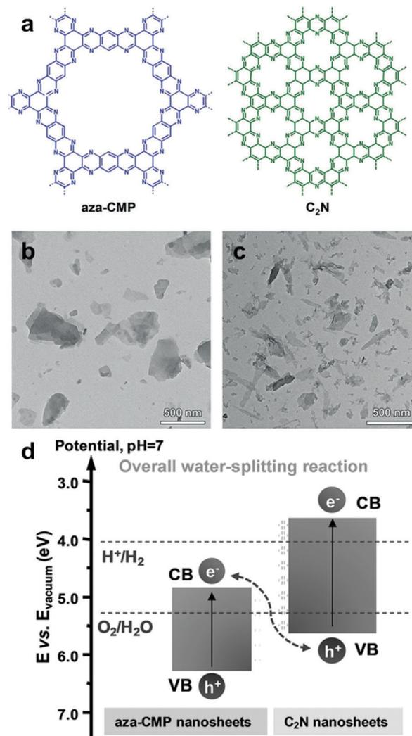
Fig. 14 Organic hybrid structure of CPPs for energy band alignment. (a) Chemical structure of aza-conjugated microporous polymer (aza-CMP) and  $C_2N$  nanosheets. TEM images of the exfoliated (b) aza-CMP and (c)  $C_2N$  nanosheet. (d) Electronic band structures of aza-CMP and  $C_2N$  nanosheet for a Z-scheme heterostructure. Reproduced with permission.<sup>111</sup> Copyright 2018 Wiley-VCH.
