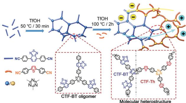
Fig. 5 Enhanced charge separation within a covalent triazine framework by creating an intramolecular heterostructure *via* sequential copolymerization strategy. Reproduced with permission.<sup>86</sup> Copyright 2018 Wiley-VCH.
