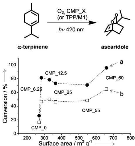
Fig. 17 Porosity control of CPPs by the silica template. Photocatalytic conversion of  $\alpha$ -terpinene into ascaridole with poly(benzothiadiazole)s having difference surface areas. Photo-reactor set-up with (a) lower  $O_2$  flow rate (5 mL  $min^{-1}$ ) and (b) higher  $O_2$  flow rate (10 mL  $min^{-1}$ ). Adapted with permission.<sup>22</sup> Copyright 2013 Wiley-VCH.
