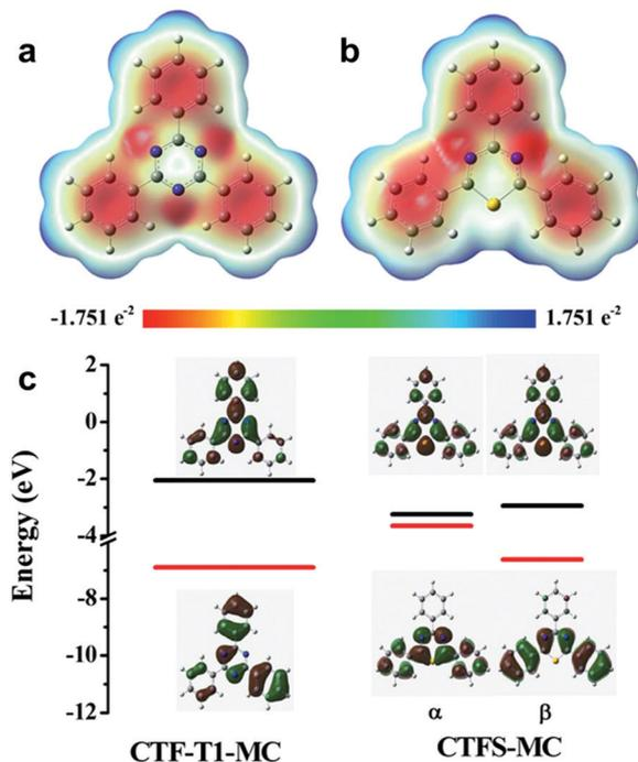
**Fig. 13** Elemental doping on CPPs for controlling the energy band structure. Charge distributions of cluster models from structures of (a) covalent triazine framework (CTF-T1-MC) and (b) sulfur-doped CTF (CTFS-MC). (c) The calculated HOMO/LUMO orbitals of the cluster models. Adapted with permission.<sup>106</sup> Copyright 2016 The Royal Society of Chemistry.
