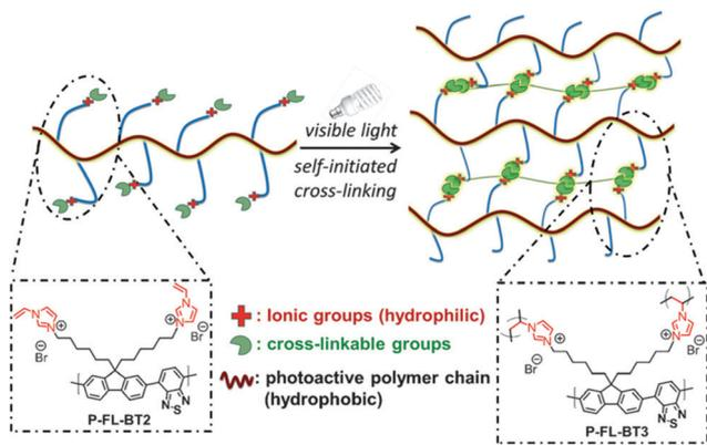
Fig. 20 Functionality control of CPPs for water compatibility. Conjugated polymer networks with vinylimidazolium group for self-initiated cross-linking. Adapted with permission.<sup>128</sup> Copyright 2015 Wiley-VCH.
