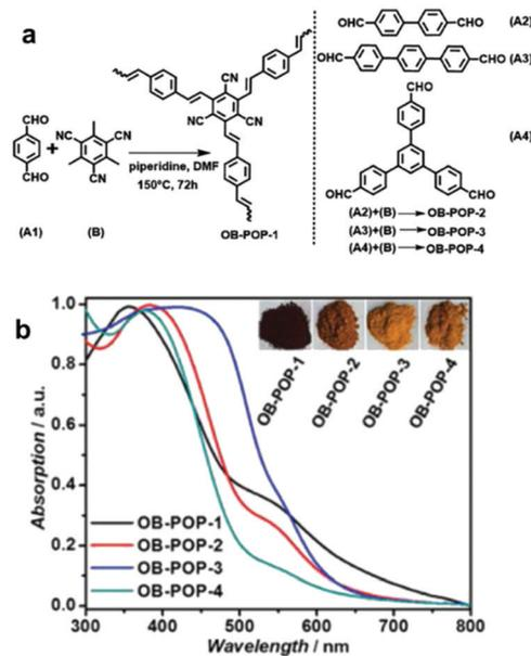
**Fig. 2** Enhanced light absorption using longer phenylene linkers in CPPs. (a) Synthetic process of olefin-bridged porous organic polymers (OB-POPs) and (b) their UV/vis diffuse reflectance spectra with photographs of the resulting polymers (inset). Reproduced with permission.<sup>27</sup> Copyright 2017 Wiley-VCH.
