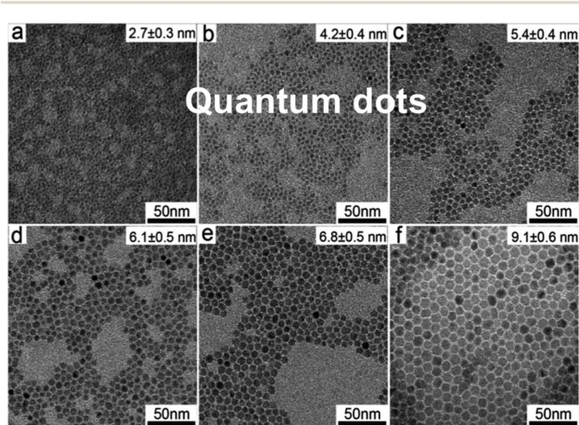
Fig. 11 S-band photoluminescent silicon nanocrystals of controllable size.<sup>188</sup> Adapted with permission from Y. Yu, G. Fan, A. Fermi, R. Mazzaro, V. Morandi, P. Ceroni, D. M. Smilgies and B. A. Korgel, *J. Phys. Chem. C*, 2017, **121**, 23240–23248. Copyright 2007 American Chemical Society.
