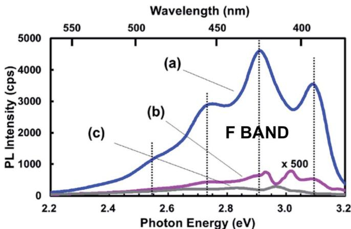
Fig. 16 Photoluminescence of adsorbed fluorescent organic contaminants on silicon nanoparticles.<sup>268</sup> Adapted with permission from T. Matsumoto, M. Maeda and H. Kobayashi, *Nanoscale Res. Lett.*, 2016, 11(7), available via an open access CC-BY license.
