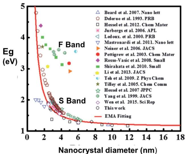
Fig. 13 Size dependence of photoluminescence for silicon quantum dots.<sup>208</sup> Reprinted with permission from X. Liu, Y. Zhang, T. Yu, X. Qiao, R. Gresback, X. Pi and D. Yang. *Part. Part. Syst. Charact.*, **33**(1), 44–52, 2016. Copyright 2015, WILEY-VCH Verlag GmbH & Co. KGaA, Weinheim. Some of the featured studies reported F-band data rather than S-band data, as highlighted here.
