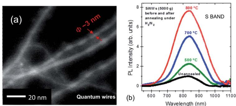
Fig. 10 Luminescent ultrathin silicon nanowires from plasma synthesis and their S-band 300 K PL at varying levels of surface passivation.<sup>184</sup> Adapted with permission from V. Le Borgne, M. Agati, S. Boninelli, P. Castrucci, M. de Crescenzi, R. Dolbec and M. A. E. Khakani, *Nanotechnology*, 2017, **28**, 285702. Copyright IOP Publishing. All rights reserved.
