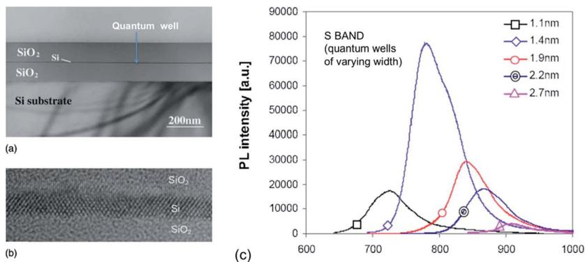
Fig. 8 Single silicon quantum well and associated S-band PL for varying well thickness.<sup>162</sup> Reprinted and adapted with permission from E. C. Cho, M. A. Green, J. Xia, R. Corkish, P. Reece, M. Gal and S. H. Lee. *J. Appl. Phys.*, 2007, **101**, 024321. Copyright AIP Publishing.
