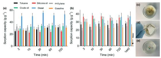
Fig. 6 The oil and solvent removal performance of the nanofibrous mat as a function of time using (a) pure oils and organic solvents, and (b) a mixture of pure oils and organic solvents with water as feed solutions. The mat was used for water adsorption as a control to show its hydrophobic nature. Optical photos for the treatment of crude oil spillage on the seawater with the 6FDA-TrMPD nanofibrous mat (c) before, (d) during, and (e) after treatment of an oil spill.
