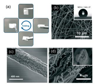
Fig. 2 (a) Optical photos showing the 6FDA-TrMPD mat during the folding/unfolding process,  $c_{\text{6FDA-TrMPD}} = 10\%$  (w/v). (b) SEM image of the nanofibers and its water wettability showing hydrophobicity. (c) SEM image of a single nanofiber showing a wrinkled texture. (d) Crosssection image of the mat and fiber (inset).
