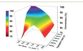
Fig. 3 3D bivariate coordinate system optimizing the TBCR. The air flow was studied in the range of 0.5 L min<sup>-1</sup> to 3.0 L min<sup>-1</sup>. The ratio of 2-propanol/water (v/v) was investigated from 10% to 60%.
