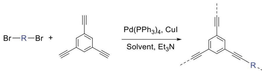
**Fig. 1** The preparation of the CMP networks formed via a palladium-catalysed Sonogashira–Hagihara reaction of 1,3,5-triethynylbenzene with an aromatic DBM.
