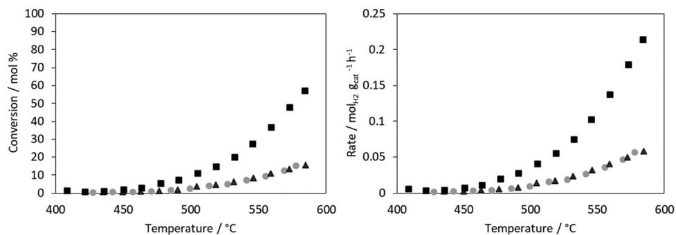
Fig. 10 Catalytic activity (left) and rate of reaction (right) of ▲ Co-aerogel (1.7 wt% Co), ● Re-aerogel (1.5 wt% Re), ■ CoRe gel (3 wt% Co–2.7 wt% Re). Reaction conditions: 2.5 mL min<sup>-1</sup> NH<sub>3</sub>, 6 mL min<sup>-1</sup> He, 25 mg catalyst, GHSV: 6000 h<sup>-1</sup>. Catalysts are pre-reduced at 330 °C under H<sub>2</sub> flow.
