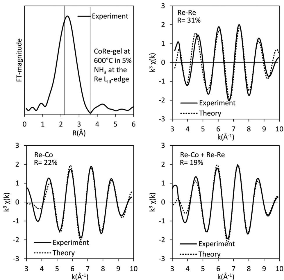
Fig. 15 Fourier filtered and fitted backscattered signal originating from metallic contribution (real space range:  $2\text{--}3.4\text{ \AA}$ ) for the CoRe-gel at  $600^\circ\text{C}$  in 5%  $\text{NH}_3$  at the  $\text{Re L}_{\text{III}}$ -edge.
