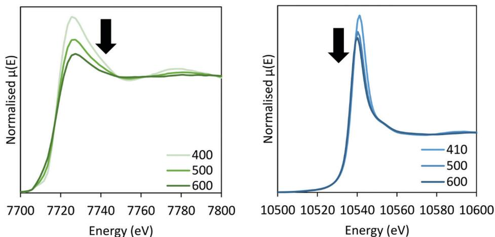
Fig. 11 XANES of the CoRe-gel during ammonia decomposition at the Co K-edge (left) and Re L<sub>III</sub>-edge (right) between 400–600 °C in 5% NH<sub>3</sub>.
