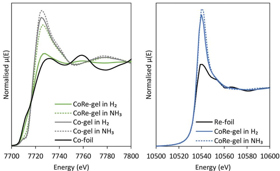
Fig. 9 XANES-spectra before and after switching from H<sub>2</sub> to NH<sub>3</sub> from the Co K-edge (left) and Re L<sub>III</sub>-edge (right).
