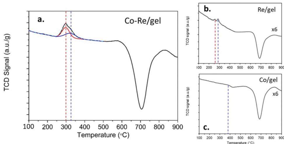
Fig. 3 Temperature programmed reduction (TPR) of the as-synthesised catalysts (a) 2.7 wt% Co–3 wt% Re on silica aerogel (CoRe/gel), (b) 1.0 wt% Re on silica aerogel (Re/gel) and (c) 2.9 wt% Co on silica aerogel (Co/gel). The TCD signal of (b) and (c) have been multiplied 6 times to show any H<sub>2</sub> consumption peaks.
