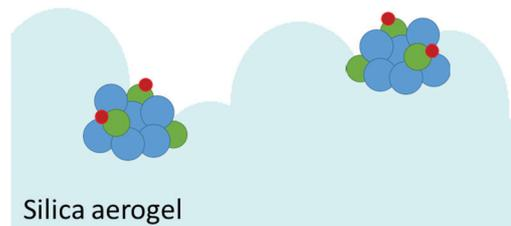
Fig. 8 Schematic of the CoRe-gel in 75% H<sub>2</sub> at 600 °C with the major species consisting of rhenium (blue), cobalt (green) and oxygen (red).
