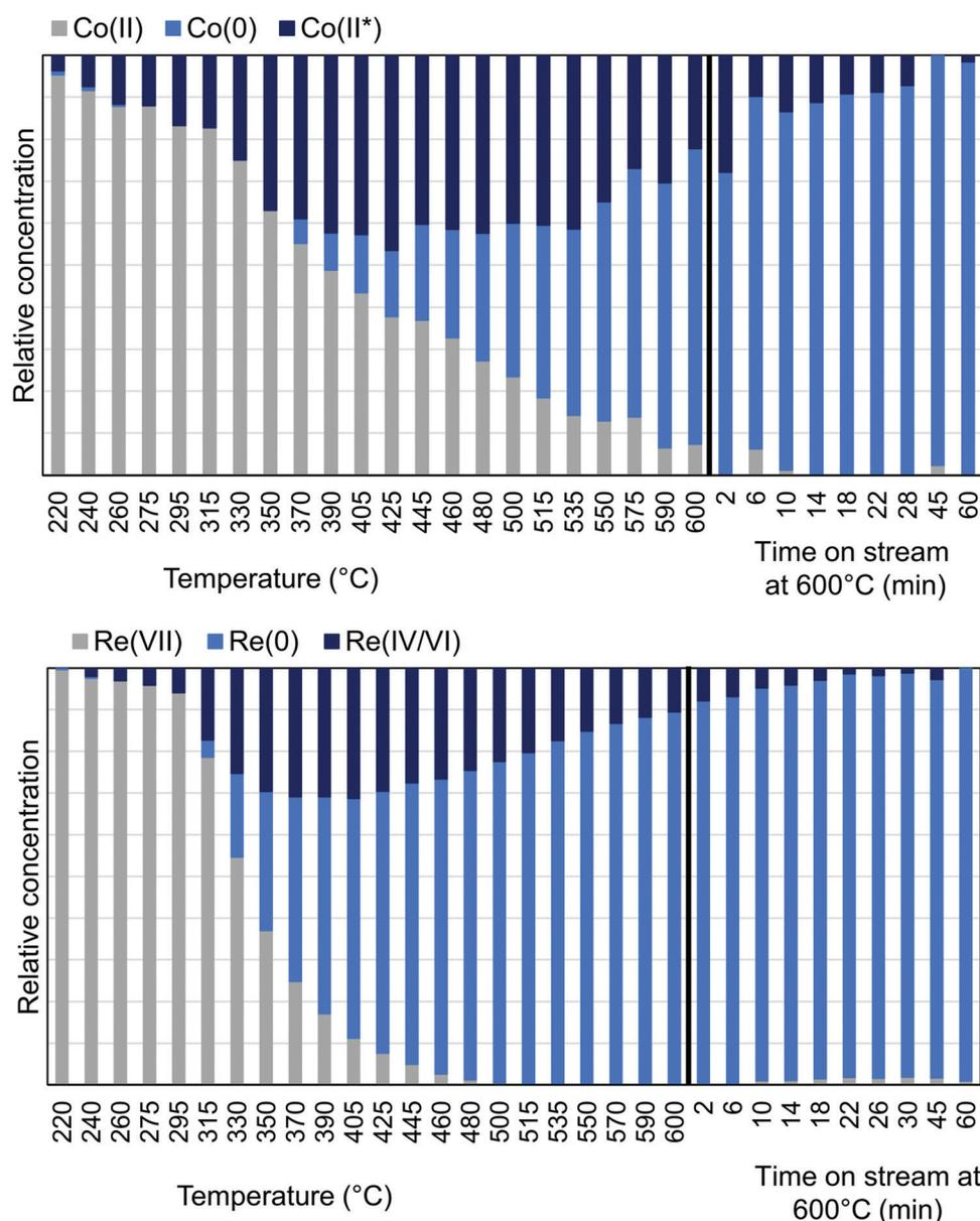
Fig. 7 MCR-analysis of the pre-treatment of CoRe-gel from the Co K-edge (top) and Re L<sub>III</sub>-edge (bottom) with the relative concentrations of the components.
