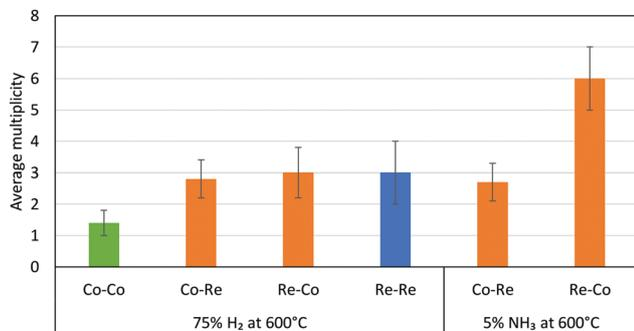
Fig. 16 Average multiplicities of the CoRe-gel after pre-treatment in H<sub>2</sub> and during ammonia decomposition. The Me–O/N shells were removed for clarification.
