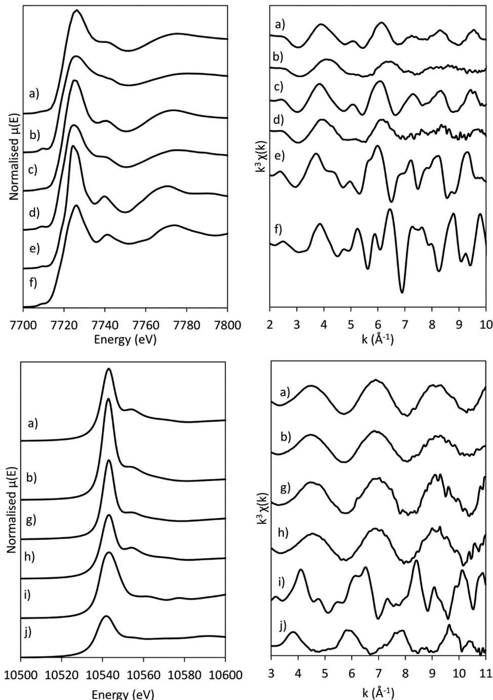
Fig. 4 XANES spectra (left) and  $k^3$ -weighted chi-curves (right) of the (a) as-synthesised CoRe-gel, (b) annealed CoRe-gel, (c) as-synthesised Co-gel, (d) annealed Co-gel, (e)  $\text{Co}(\text{OH})_2$ , (f)  $\text{CoO}$ , (g) annealed Re-gel, (h)  $\text{NH}_4\text{ReO}_4$ , (i)  $\text{ReO}_3$  and (j)  $\text{ReO}_2$  at the Co K-edge (top) and at the Re  $L_{\text{III}}$ -edge (bottom).
