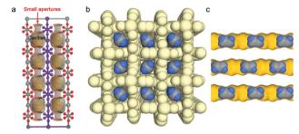
**Fig. 10** Schematic illustrations of pore size-controlled uptake of (a)  $C_2H_2$  in **SIFSIX-14-Cu-i**; <sup>42</sup> (b and c)  $C_2H_4$  in UTSA-280.<sup>57</sup> (Reprinted with permissions from ref. 42 and 57: copyright 2017, Wiley-VCH Verlag GmbH & Co. KGaA, Weinheim; copyright 2018, Springer Nature.)
