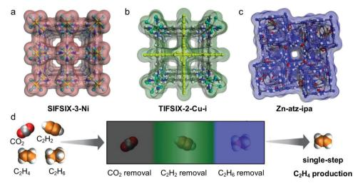
Fig. 15 (a-c) 1D ultramicroporous channels in the pcu topology PCN sorbents (a) SIFSIX-3-Ni, (b) TIFSIX-2-Cu-i and (c) Zn-atz-ipa, respectively; (d) SSST to purify  $C_2H_4$  in one-step from a  $CO_2/C_2H_2/C_2H_4/C_2H_6$  quaternary gas mixture.
