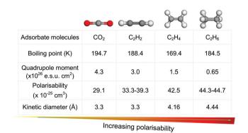
Fig. 2 Comparison of key physicochemical properties of CO<sub>2</sub> and C2 LHs reveals the similarities in properties for multiple industrially relevant gas pairs.
