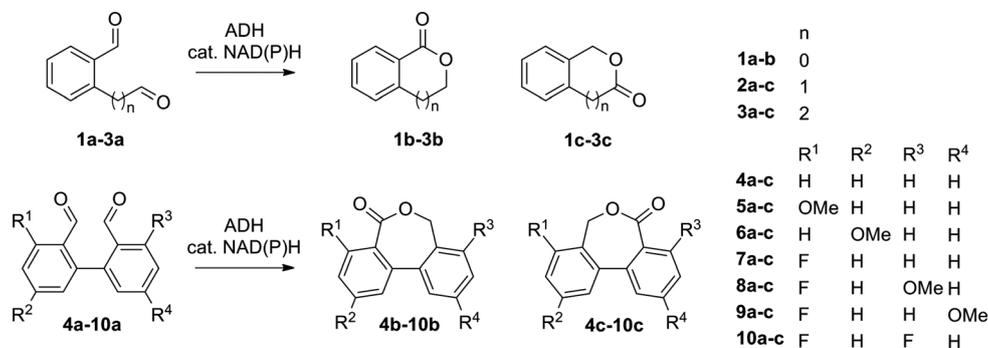
**Scheme 2** Conversion of **1a–10a** into two possible regioisomers **1b–10b** and **1c–10c** in the intramolecular Tishchenko-like reaction catalyzed by alcohol dehydrogenase (ADH). The cofactor NAD(P)H is added in catalytic amounts.
