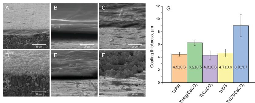
Fig. 3 SEM images of cross-sections of bare Ti (A) and coated Ti: Ti-Alg (B), Ti-Alg-CaCO<sub>3</sub> (C), Ti-CaCO<sub>3</sub> (D), Ti-DS (E), and Ti-DS-CaCO<sub>3</sub> (F); the average thickness of these coatings (G).
