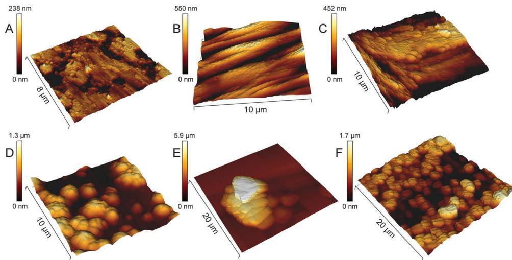
Fig. 5 AFM topography of Ti surfaces: unmodified (A), and coated with  $\text{Ca}^{2+}$ -crosslinked Alg hydrogel (Ti-Alg) (B); Ti surface coated with dextran sulfate (Ti-DS) (C); Ti surface mineralized with  $\text{CaCO}_3$  (Ti- $\text{CaCO}_3$ ) (D); Ti surface coated with  $\text{CaCO}_3$ -mineralized  $\text{Ca}^{2+}$ -crosslinked Alg hydrogel (Ti-Alg- $\text{CaCO}_3$ ) (E); and Ti surface coated with  $\text{CaCO}_3$ -mineralized dextran sulfate (Ti-DS- $\text{CaCO}_3$ ) (F).
