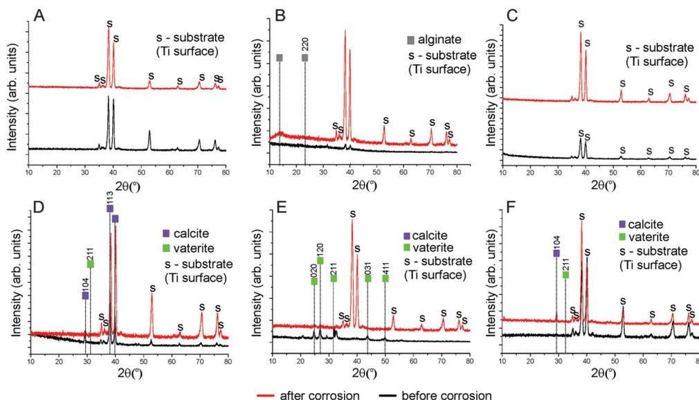
Fig. 6 X-ray diffractograms of the bare Ti surface (A); Ti surface coated with  $\text{Ca}^{2+}$ -crosslinked Alg hydrogel (Ti-Alg) (B); Ti surface coated with dextran sulfate (Ti-DS) (C); Ti surface mineralized with  $\text{CaCO}_3$  (Ti- $\text{CaCO}_3$ ) (D); Ti surface coated with  $\text{CaCO}_3$ -mineralized  $\text{Ca}^{2+}$ -crosslinked Alg hydrogel (Ti-Alg- $\text{CaCO}_3$ ) (E); and Ti surface coated with  $\text{CaCO}_3$ -mineralized dextran sulfate (Ti-DS- $\text{CaCO}_3$ ) (F).
