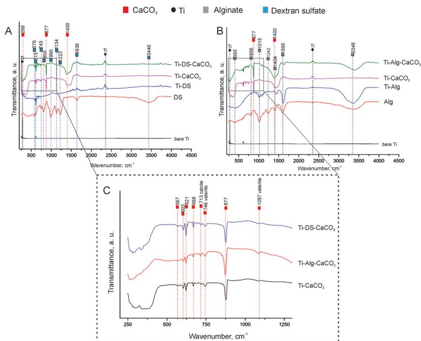
Fig. 4 ATR-FTIR spectra of the bare Ti surface and Ti surfaces with modifications: (A) spectra of Ti-DS, Ti-DS-CaCO<sub>3</sub>, Ti-CaCO<sub>3</sub> and dextran sulfate powder; (B) spectra of Ti-Alg, Ti-Alg-CaCO<sub>3</sub>, Ti-CaCO<sub>3</sub> and Ca<sup>2+</sup>-crosslinked Alg hydrogel; and (C) spectra of mineralized Ti surfaces (Ti-CaCO<sub>3</sub>, Ti-Alg-CaCO<sub>3</sub>, Ti-DS-CaCO<sub>3</sub>) in the wavenumber range 250–1300 cm<sup>-1</sup>.
