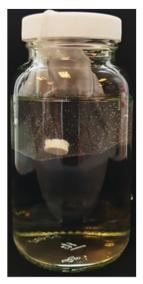
Fig. 4 PNA65-50 cylindrical aggregate nanogel implant held inside 150 μm pore size mesh bag suspended in release media.
