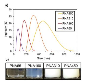
Fig. 2 PolyNIPAm nanogels synthesised in a range of sizes (a) DLS size distribution by intensity at 25 °C for each nanogel as a 1 mg mL<sup>-1</sup> aqueous dispersion, (b) nanogel dispersion turbidity as a 15 mg mL<sup>-1</sup> aqueous dispersion at 25 °C.
