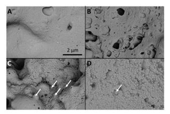
The four different nanogel aggregates with SDNs at 50% loading. (A) PNA65, (B) PNA160, (C) PNA310, (D) PNA 450. The arrows indicate lopinavir SDNs. The scale bar corresponds to all images.
