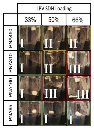
Fig. 6 Images of in vitro release nanogel aggregate drug implants after 360 hours. The mechanical stability of the implants is categorised into (I) retains shape with no fracturing. (II) a low number of fractures occur. where ca. <10% of the implant volume may separate into a small number of fragments, (III) a high number of fractures occur so that the implant separates into many fragments (ca. >10% of the implant volume).
