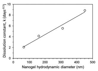
Fig. 7 Comparison of dissolution constant (k) for mechanically stable aggregate implants (PNA65) and implants which fracture during release at increased loading % (PNA160, PNA310, PNA450).
