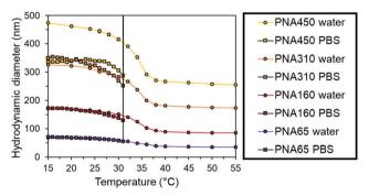
Fig. 3 Hydrodynamic diameter of nanogels in water (circles) and PBS (squares) measured using DLS at 1 mg  $\,\mathrm{mL}^{-1}$  with respect to the nanogel concentration. All the nanogels sample in PBS aggregated at 31 °C and produced particles sizes that could not be accurately measured by DLS. This behaviour is indicated by the vertical line at 31 °C for nanogel samples in PBS
