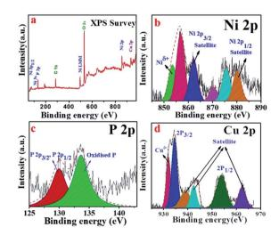
Fig. 4 (a) XPS survey spectra of Cuf@Ni<sub>5</sub>P<sub>4</sub>, and high-resolution deconvoluted XPS sspectra for: (b) Ni 2p; (c) P 2p; and (d) Cu 2p.
