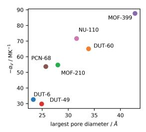
Fig. 3 The observed correlation between mesopore size and volumetric coefficient of expansion,  $\alpha_{\rm V}$ .
