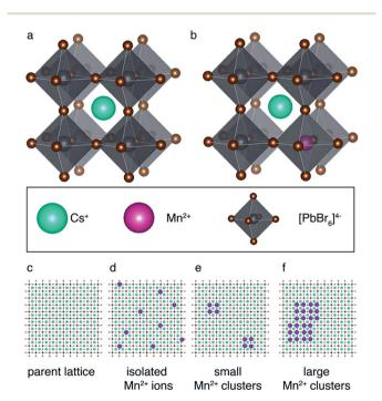
Fig. 1 Schematic representation of paramagnetic doping in perovskites: (a) parent  $CsPbBr_3$  lattice, (b) homovalent B-site replacement. Schematic representation of possible scenarios for  $Mn^{2+}$  aggregation inside the perovskite lattice: (c) parent perovskite lattice, (d) isolated  $Mn^{2+}$  ions, (e) small  $Mn^{2+}$  clusters, (f) large  $Mn^{2+}$  clusters.
