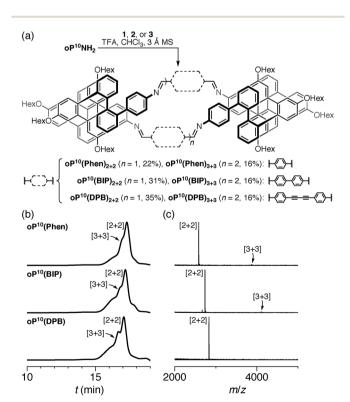
Fig. 6 (a) Assembly of  $oP^{10}(NH_2)$  with linkers 1, 2, and 3. (b) GPC chromatograms of the (quenched) crude reaction mixtures after 11 d (RI detection). (c) MALDI mass spectra of the crude reaction mixtures.
