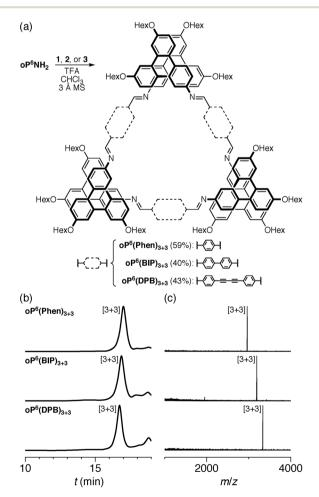
Fig. 1 (a) Assembly of  $oP^6(NH_2)$  with linkers 1, 2, or 3. (b) GPC chromatograms of the (quenched) crude reaction mixtures after 5 d (RI detection). (c) MALDI mass spectra of the crude reaction mixtures.
