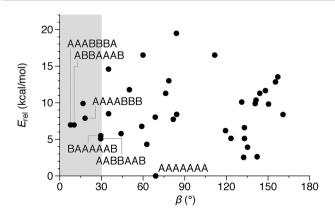
Fig. 7 Calculated  $E_{\rm rel}$  vs.  $\beta$  for all conformers of deca(o-phenylene) (PCM(CHCl<sub>3</sub>)/B97-D/cc-pVDZ). Selected conformations are labeled.
