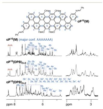
Fig. 8  $^{1}$ H NMR spectra (500 MHz, 0  $^{\circ}$ C) of  $oP^{10}(M)$ ,  $oP^{10}(DPB)_{2+2}$ , and oP<sup>10</sup>(DPB)<sub>3+3</sub>. <sup>1</sup>H assignments for the major conformers are shown (blue). For  $\mathrm{oP^{10}(DPB)_{2+2}}$ , the assignments that are grouped together are listed in order from least- to most-shielded; chemical shifts for a minor conformation were also assigned (not shown).
