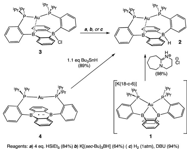
Scheme 1 Synthesis of Au(B<sub>2</sub>P<sub>2</sub>)H from H<sup>-</sup>, H<sup>+</sup>, and H<sup>+</sup>.
