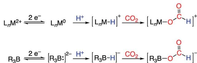
Fig. 1 Redox-coupled hydride formation at a transition metal complex (top) and borane (bottom) as a strategy for CO<sub>2</sub> electro-reduction to formate.
