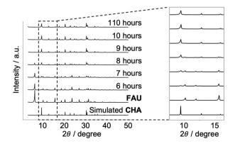
Fig. 2 Powder X-ray diffraction patterns of the starting FAU and recovered samples with different heating times together with the simulated patterns for CHA.
