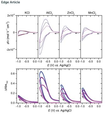
Fig. 6 (Top) Cyclic voltammograms and (Bottom) cyclic voltabsorptograms (monitored at 780 nm) at a GLAD-TiO $_2$ /TiO $_2$ /ITO electrode immersed in different aqueous electrolytes (adjusted to pH 3.0) made of (from left to right): 0.3 M KCl, 0.25 M AlCl $_3$ , 0.25 M ZnCl $_2$ , or 0.25 M MnCl $_2$ . Currents are expressed in flux density normalized to the scan rate. Scan rates: (blue) 0.1, (purple) 0.2, and (magenta) 0.5 V s $^{-1}$ . The potential is quoted vs. Ag/AgCl.
