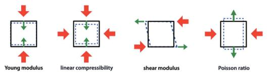
Fig. 1 Representation (from left to right) of Young's modulus (E), linear compressibility (B), shear modulus (B), and Poisson's ratio (B), four directional elastic properties of crystalline materials. Red arrows represent the direction of stress exerted, while green ones represent the axis along which the response is measured. Reproduced from ref. 10 with permission. Copyright 2016 IOP Publishing Ltd.
