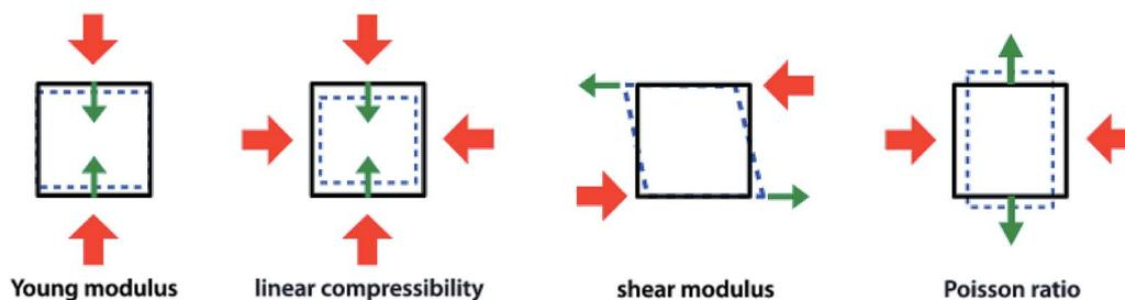
Fig. 1 Representation (from left to right) of Young's modulus ( $E$ ), linear compressibility ( $\beta$ ), shear modulus ( $G$ ), and Poisson's ratio ( $\nu$ ), four directional elastic properties of crystalline materials. Red arrows represent the direction of stress exerted, while green ones represent the axis along which the response is measured. Reproduced from ref. 10 with permission. Copyright 2016 IOP Publishing Ltd.
